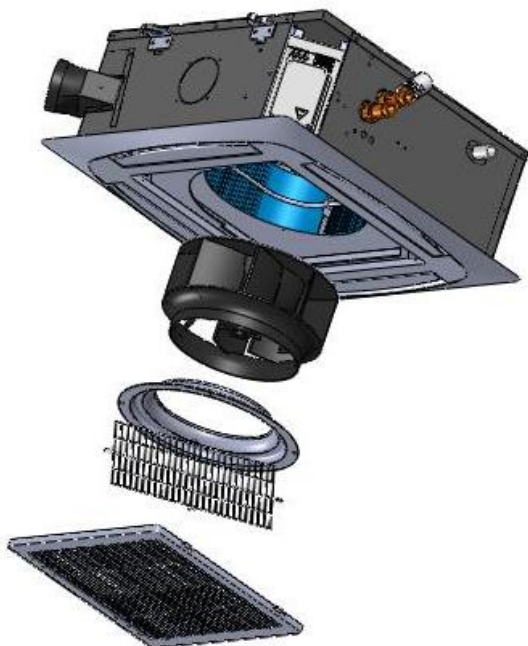
Figure 33 Step 4 : Use a spanner to remove the fan blower.
