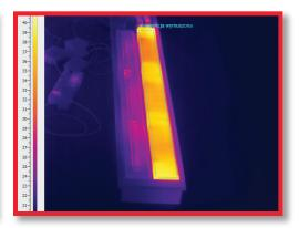
Airspeed analysis is one of the basic parameters that influence the heating power of our products. By measuring the distribution of airspeeds, we can eliminate detrimental operational factors common to trench heaters, such as the appearance of zones with very low airspeed and the cycling of already heated air.
